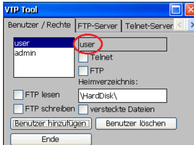
Figure 18 VTP Tool - Change of user authorization
